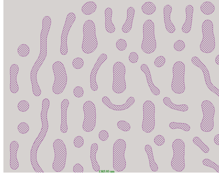
Constructed mask shapes with assist features using digital twin
